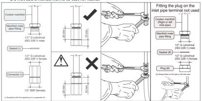
Figure 11b Connecting the gas
